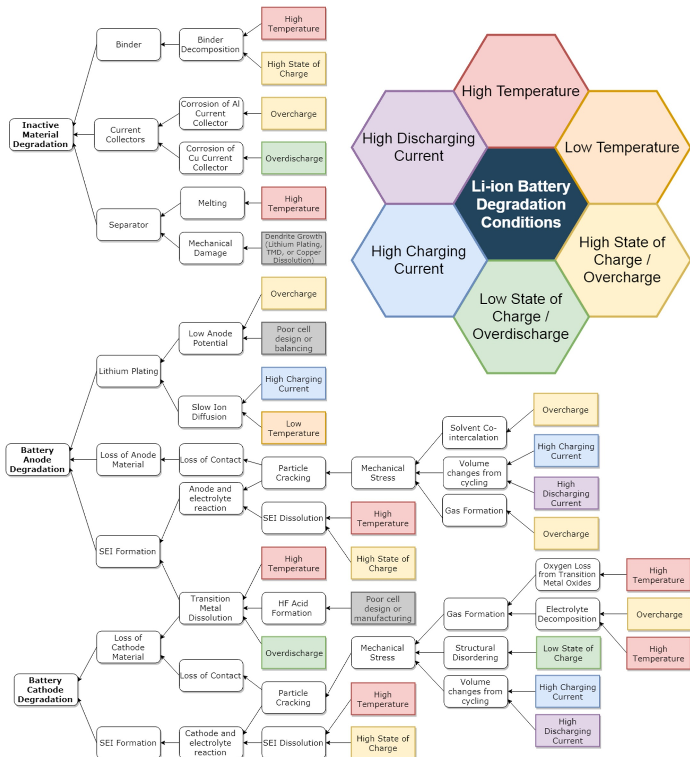
Fig. 2. Degradation mechanisms in Li-ion batteries.
